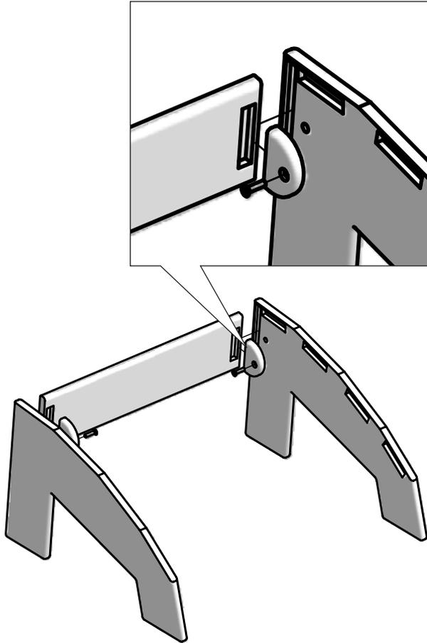
Place Back Plate between Legs and fit into cut outs. Place blocks in Back Plate cut outs and insert bolts through block into Legs and finger tighten.
