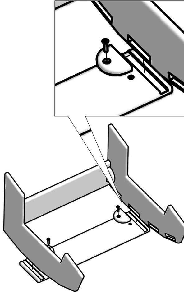
Align groove track cut outs of Middle Slat with Legs. Place blocks in Leg cut outs. Align hole in block with hole in Middle slat and insert bolt through block into Middle slat and finger tighten. Repeat this step for second Middle slat.
