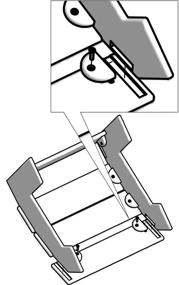
Align groove track cut outs of End Slat with Legs. Place blocks in Leg cut outs. Align hole in block with hole in End slat and insert bolt through block into End slat and finger tighten. Repeat this step for opposite End slat. **Using provided wrench securely tighten all bolts.**
